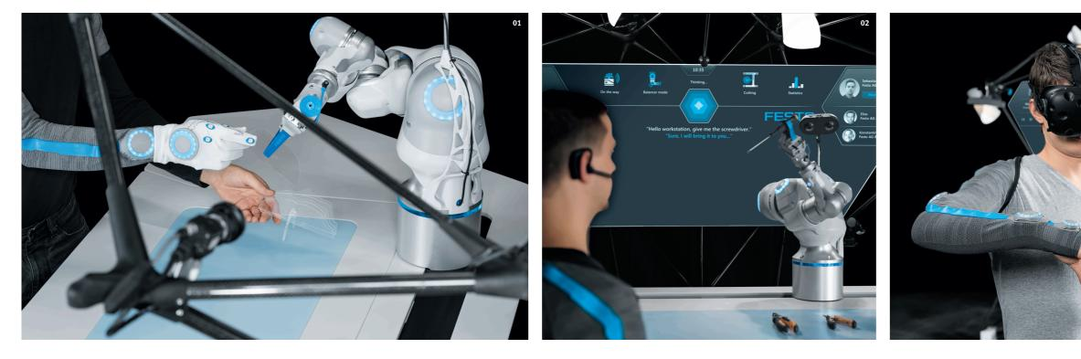
The worker's special work clothing consists of a long-sleeved top, which is equipped with inertia sensors, and a work glove with integrated infrared markers. All the necessary cables are integrated in the fabric of these so-called wearables, so that they do not hinder the worker's movements.
