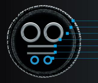
Sensor glove 3D textile knitted fabric Rubber bellows Tubing connection Leaf spring Bending sensor Two structural elements
