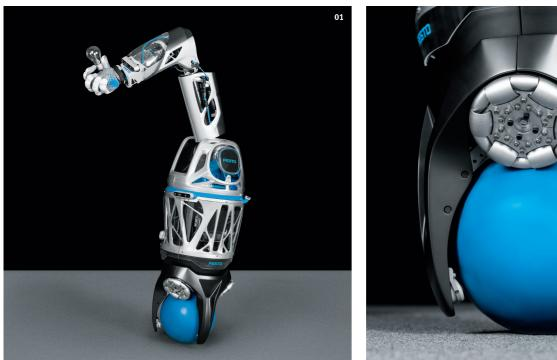
For the BionicMobileAssistant, the BionicSoftHand 2.0 is combined with a mobile ballbot and a lightweight, electric robot arm – the DynaArm. Thanks to model-based force control and control algorithms to compensate for dynamic effects, the arm can react well to external influences and thus interact very sensitively with its environment.
