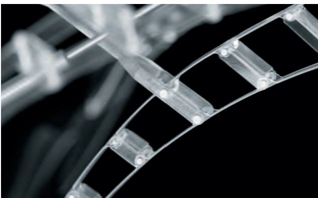
Bionic transfer: the Fin Ray® structure in the AquaJelly tentacles ...
