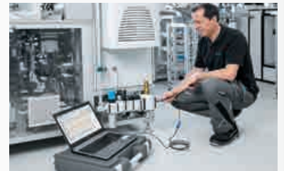
Analysis of compressed air distribution
