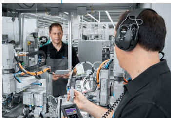
Leakage detection and elimination
