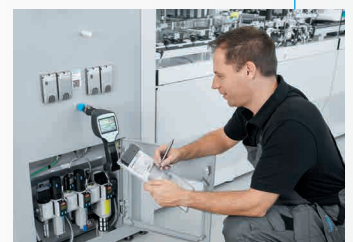
Compressed air quality analysis
