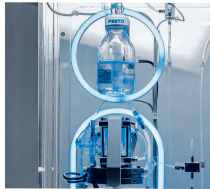
Electrolysis: production of hydrogen from water.
