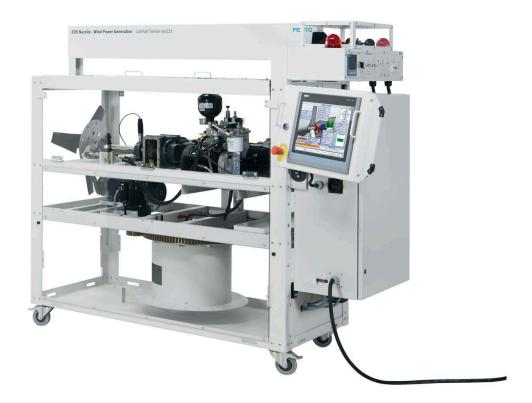
The Nacelle - Wind Turbine Learning System is a complete scaled-down version of commercial wind turbine nacelles, making it an excellent substitute for expensive actual equipment. Space efficient and affordable the machine fully interacts with users, thus enhancing the learning experience.
