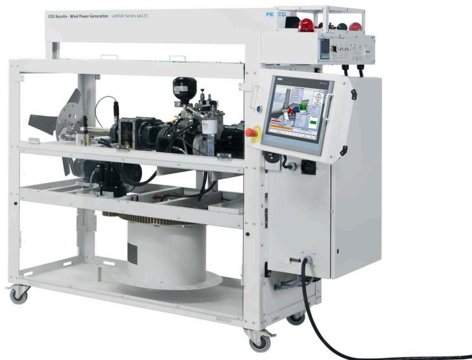
The Nacelle - Wind Turbine Learning System is a complete scaled-down version of commercial wind turbine nacelles, making it an excellent substitute for expensive actual equipment. Space efficient and affordable the machine fully interacts with users, thus enhancing the learning experience.
