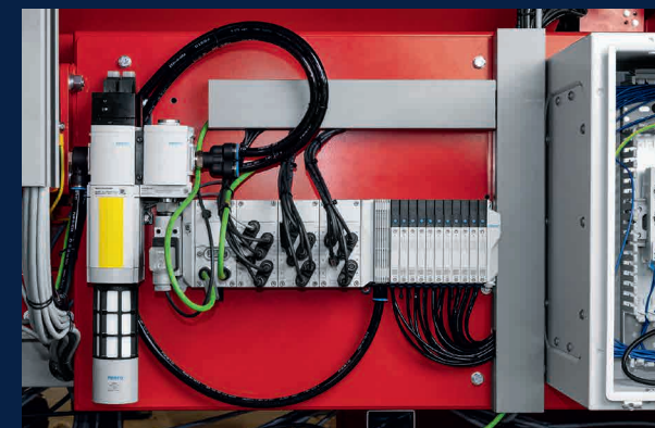
The special feature of the valve terminal VTUX: It is suitable for both decentralized and centralized machine installation. At Aventec, they opted for decentralized control.
