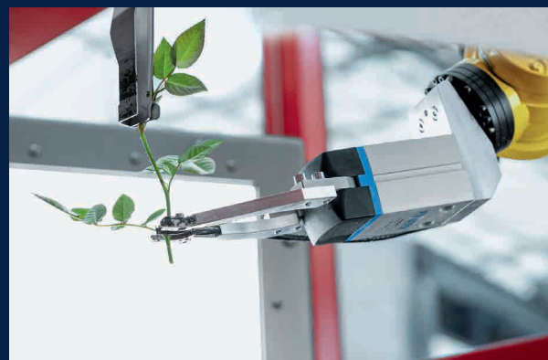
Fully automated filigree work: The new machine from Aventec cuts and plants up to 5,200 rose cuttings per hour using Festo components.
