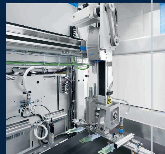
A handling system with electric axes EGC and ELCC ensures the finished blister packs are reliably transported.
