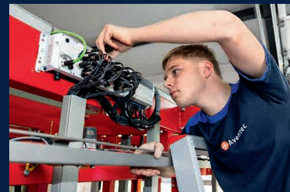
The special feature of the valve terminal VTUX: It is suitable for both decentralized and centralized machine installation. At Aventec, they opted for decentralized control.
