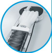
HASEL actuator (Hydraulically amplified self-healing electrostatic)
