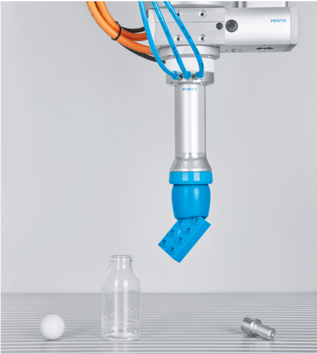
Gripping with controlled pneumatics
