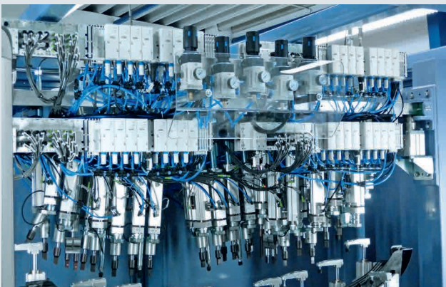
Maximum functionality – minimal space requirements: VPPM-MPA integrated into the electrical terminal CPX/MPA
