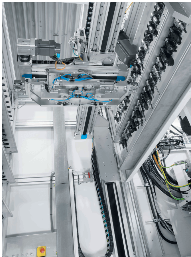
Tool changer reduces setup times: this tandem gripper/rotary unit comprises axes EGC, the pneumatic semi-rotary drive DRRD and the heavy-duty tool gripper HGPT and is a complete and ready-to-install handling solution from Festo. Photo: Festo
