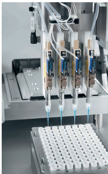
The automated pipetting system , consisting of the pipetting head DHOE and the disposable syringe ejector DHAO can accurately dispense volumes in the range of 10 µl.
