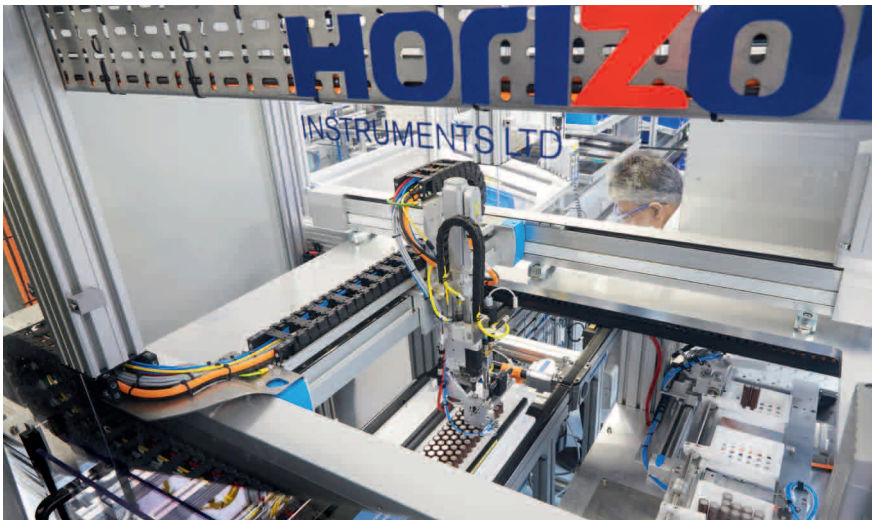
Automation solutions specialist Horizon Instruments designed and integrated the Festo planar surface gantry.
