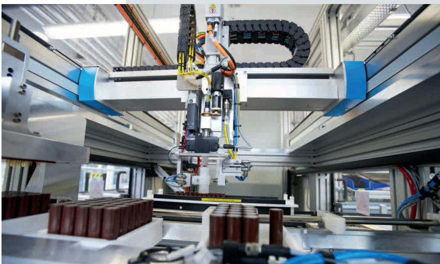
High-speed battery cell pick & place with the planar surface gantry EXCH from Festo.
