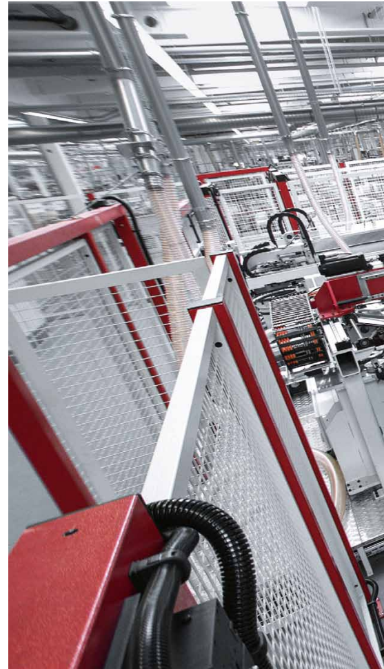
Automation technology from Festo is responsible for moving the front panels and drawers from one assembly step to the next as well as for secure holding and clamping.
