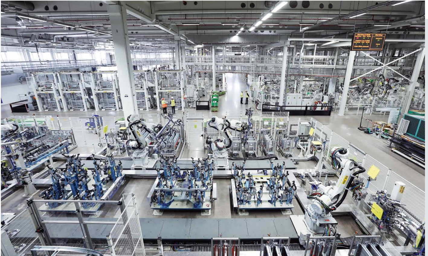
At the Scania body shop in Oskarshamn, 288 robots weld truck cabs together.
