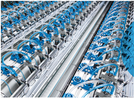
Gentle placement of large metal sheets from a transport system to a stack by multiple cylinders
