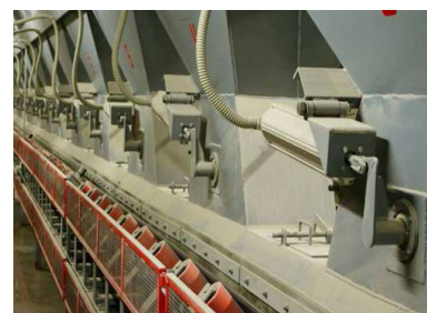
Silo emptying control in the manufacture of fertilisers
