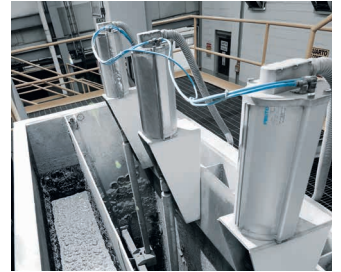
Control of dart valve for level regulation in mineral processing
