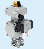
Quarter turn actuator DFPD, ball valve VZBE, pilot valve VSNC, sensor box SRBC
