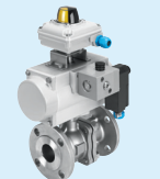
Quarter turn actuator DFPD, ball valve VZBF, pilot valve VOFC, sensor box SRBC
