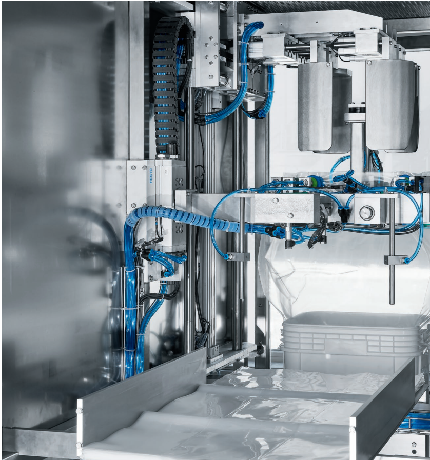
Bag in a box: a handling system uses a vacuum gripper to remove the bags from a feed magazine, which are then inflated before being inserted in a pre-prepared box.
